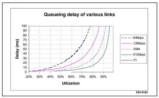
As can be seen in Figure 18, queueing delays can be significant for links with bandwidth under 512 kbit/s, whereas with higher speed links they can tolerate much higher utilization levels.
